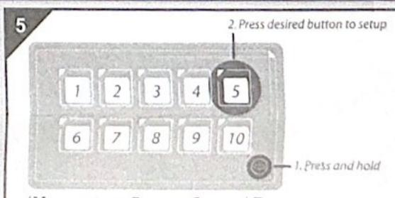
(Momentary Button Set-up) To set up a specific button to be momentary (Push-On), press and hold the backlight button to enter setup mode (white backlights will be blinking). Press the desired button to enable momentary function on it, press again to disable. The ON-indicatigon LED will be blinking for Momentary buttons and stays ON for normal buttons during setup mode. Release the backlight button to exit setup mode.
